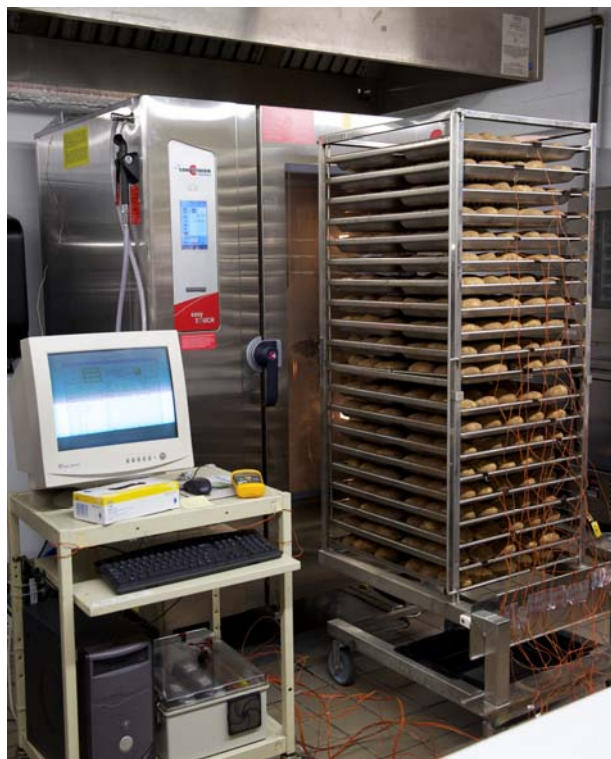
Figure 7: Rack-trolley Instrumented for Convection Mode Testing
