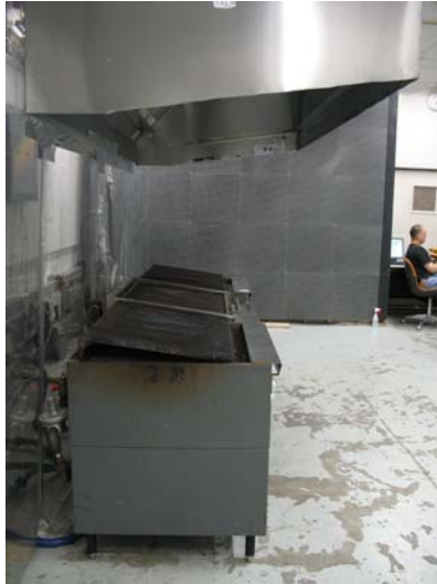
Figure 3. Side View of Set Up Without Standard 45-inch by 45-inch by 45° Side Panels
